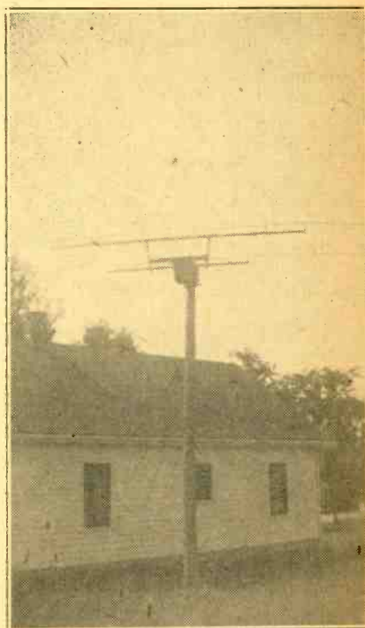
D—The W1CBV antenna, a two-element rotary beam, entirely home-made except the elements and the motor that turns it.
